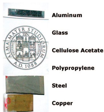
FIGURE 3. Hybrid H-DLLA50 cast on different substrates. Application on transparent substrates outlines a coating transparency to visible light.
